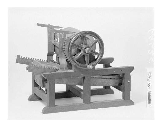
B) Flat to cylinder or plane surface to cylinder- these groups of letterpress machines are known as flat bed cylinder presses. The surface of the printing surface remains flat while the surface carrying paper is cylindrical. Earlier these presses were operated by steam power. But now days they are operated by electrical power.
